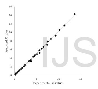
**Figure 4** Comparison of experimental values of *K* with the predicted values, obtained using equation 14
