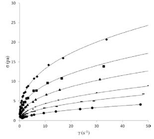
**Figure 1** Rheogram of Gum Cordia solution (20kgm<sup>-3</sup>) at different temperature (°C)
