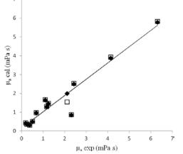
Figure 8 Comparison of predicted with experimental apparent viscosity for equa-
