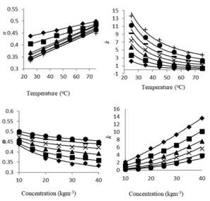
**Figure 2** Variation of *K* and *n* with concentration (kgm<sup>-3</sup>) ( $\bullet$  10  $\blacksquare$  15  $\blacktriangle$  20  $\times$  25 - 30  $\bullet$  35 + 40 ) and Temperature °C( $\bullet$  25  $\blacksquare$  35  $\bigstar$  45  $\times$  55 - 65  $\bullet$  75 ).
