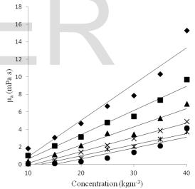
**Figure 7** Apparent viscosity as function of Concentration (kgm<sup>-3</sup>) and Temperature (°C)
